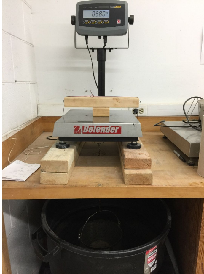
Figure 3-6: Mass of suspended concrete samples submerged in water per ASTM C642.
