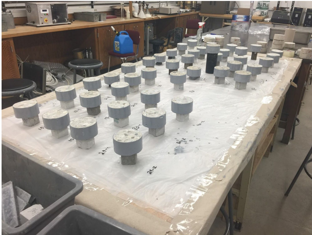
Figure 3-11: Epoxied samples in preparation for proposed RCIP testing
