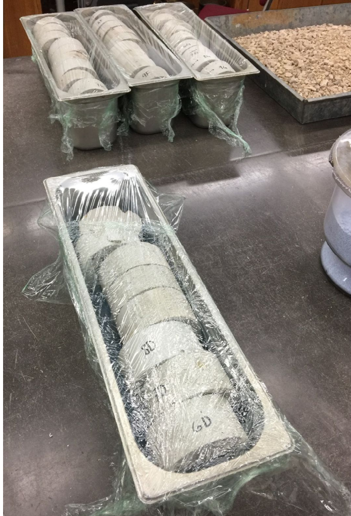
Figure 3-5: Oven-dried concrete samples sitting inside stainless-steel containers sealed with saran wrap which was secured with tap underneath the lip of the containers.
